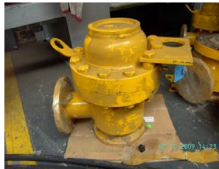
Line protection valve
