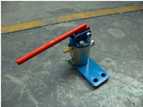
Hydro power control valve
