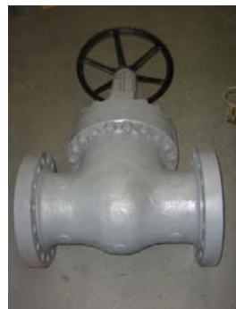
Gate valve repairs
