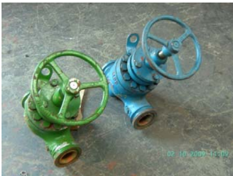
Globe & safety isolation valve repairs
