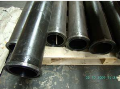
Hydro power piping (hub connection)
